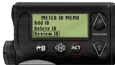
13. Select **Review ID** on your compatible Medtronic device to confirm that your **CONTOUR®NEXT LINK** meter ID has been correctly entered. If incorrect, go back to Step 10.
