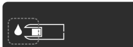
1. If the meter beeps twice and the screen displays a blinking blood drop, the test strip does not have enough blood.
