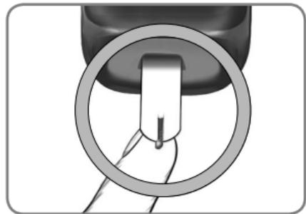
3. Hold the tip of the test strip in the blood drop until the meter beeps.
