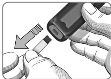
2. To turn the meter off, remove the test strip.
