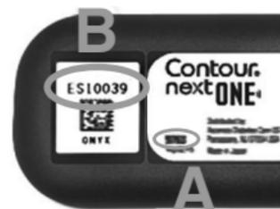
2. Locate the model number (**A**) and serial number (**B**) on the back of the meter.
