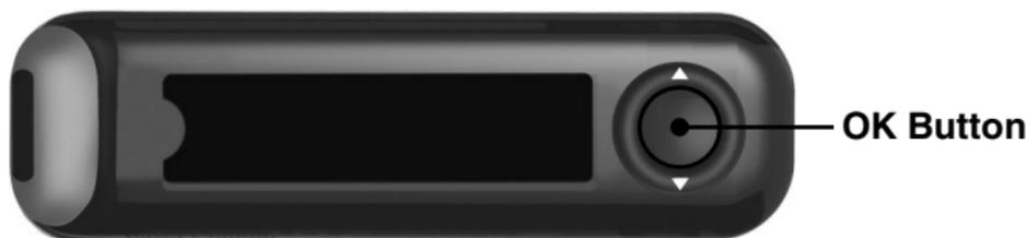
Press and hold **OK** for 3 seconds until the meter turns on.
