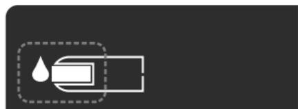
The screen displays the blinking blood drop indicating it is ready to test a blood drop.
